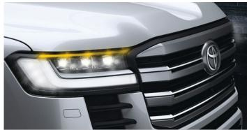
**LED HEAD LAMPS** with Sequential Turn Signal
